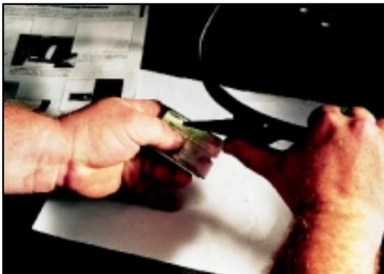
3. Gaff tip profile should be 1/4" or (.250) radius. The CCA radius is .450. Use 6303 gaff gauge for pole gaffs and the 6306 for tree gaffs.
