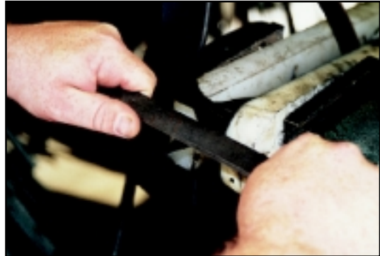
2. File gaff from heel to tip in a smooth over and down motion. Hint - color in gaff with black marker to ensure you are taking material off evenly. Never file across or against the grain as it creates stress risers which may cause gaff to break. Never file the beehive of gaff.
