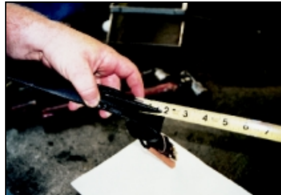
4. Never use a pole gaff shorter than 1 1/4" long. Never use a tree gaff shorter than 2 1/4" long.
