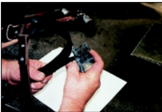
5. Check gaff width and thickness at the 1/2" and 1" windows as illustrated in the instructions included with the gaff gauge.
